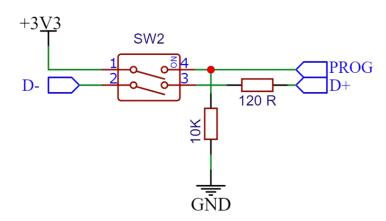
PMM0648M can be alternatively switched between two preprogrammed modes through the second dip switch.
